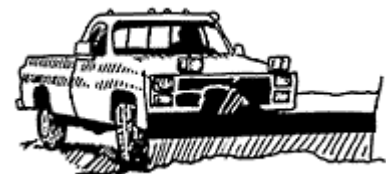
Figure 4. An even flow of snow over the blade makes snow removal more efficient and safer.
