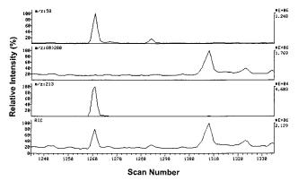
**Figure 3.** Mass chromatograms of (a) m/z 58, (b) m/z 60–200, (c) m/z 213, and (d) the reconstructed ion chromatogram for the GC peak (scan 1261) corresponding to *N*,*N*-dimethyl-1-dodecanamine. The chromatograms are from an EI analysis of three handled glass beads.
