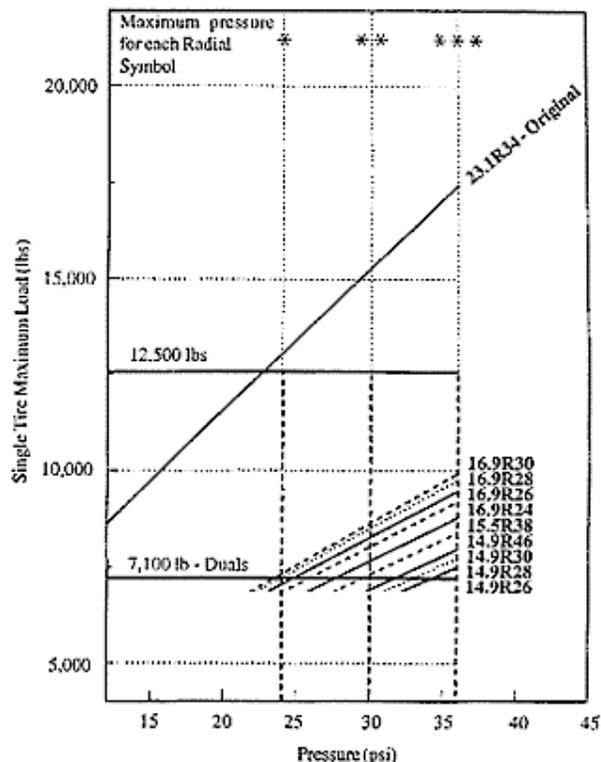
**Figure 4.** Example of using the radial tire load and inflation pressure chart to select substitute tires that can be used as straddle duals will have a narrower footprint.
