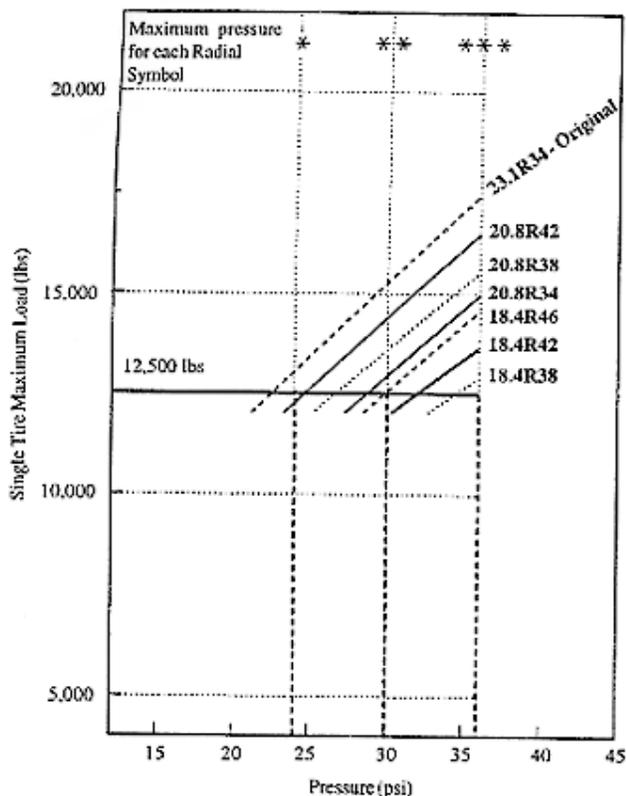
**Figure 3.** Example of using the radial tire load and inflation pressure chart to select a substitute tire that will have a narrower footprint.
