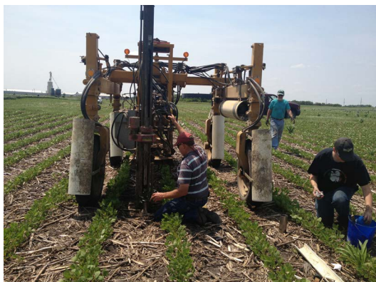
Researchers taking soil samples with a deep probe. (Photo courtesy Andrea Basche)
