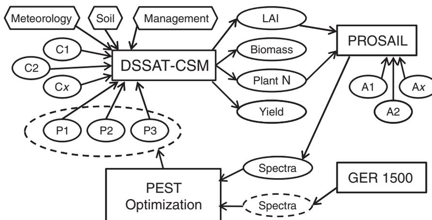
**Fig. 1.** Model inversion using a linked ecophysiological model (DSSAT-CSM) and radiative transfer model (PROSAIL). The Parameter ESTimation (PEST) algorithm was used for adjusting the DSSAT-CSM parameters for leaf area growth potential (P1, P2, and P3) to minimize error between measured and simulated canopy spectral reflectance. DSSAT-CSM simulated LAI and plant nitrogen (N) provided information to PROSAIL for spectral reflectance simulations.
