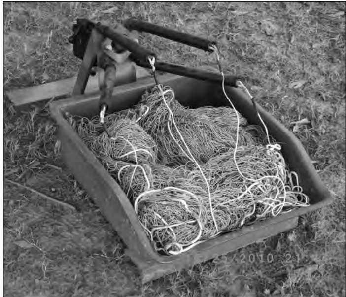
Figure 1. The basic Coda Netlauncher® configuration with net loaded in the fiberglass tray.
