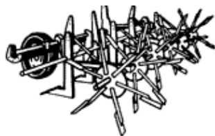
Figure 4. Implanted reservoir tillage implement and soil surface ponding.
