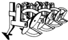
Figure 3. Basin tillage implement mounted on a cultivator and soil surface ponding conditions.
