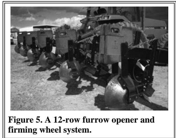
**Figure 5. A 12-row furrow opener and firming wheel system.**
