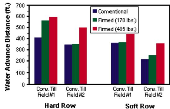
**Figure 3. Furrow advance distance in hard and soft furrows for conventionally prepared furrows, furrows firmed with Eversman v-wheel (170 lbs.) and furrows firmed with Eversman v-wheel with 485 pounds total weight.**
