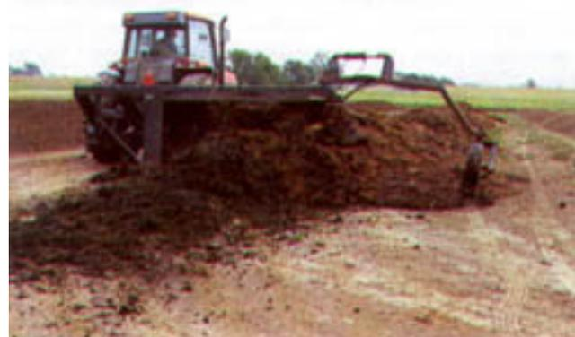
Figure 1. Turning of a composting windrow.
