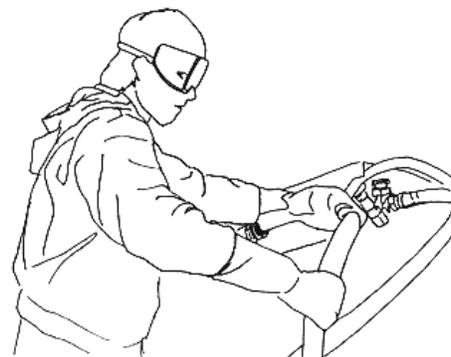
**Figure 4. Hoses are the weakest link in the anhydrous ammonia application system. Always inspect the transfer and filler hoses thoroughly. If the braided layers show through, or if kinks, bulges or coupling slippage is evident, replace as soon as possible.**
