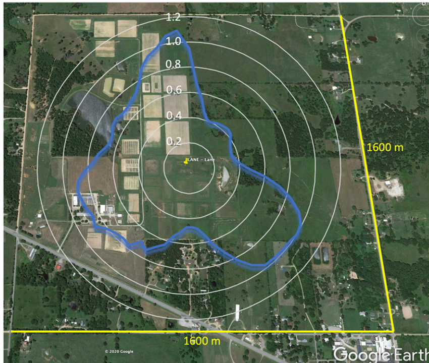
FIG. 4. Average wind speed at the Oklahoma Mesonet station in Lane normalized by the statewide average wind speed as a function of wind direction. Wind speeds from the south have magnitudes that are approximately 45% of the statewide average wind speed, and wind speeds from the southeast are approximately equal to (or 100% of) the statewide average wind speed. Areas of trees 200–500 m away are present in any direction where wind speeds are diminished.
