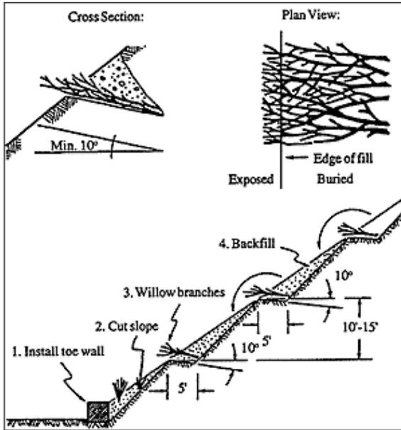
**Figure 2. Installation of brush layering. Numbered sequence of operations is shown. Vertical spacing depends on slope angel. (From Gray and Leiser, 1982)**
