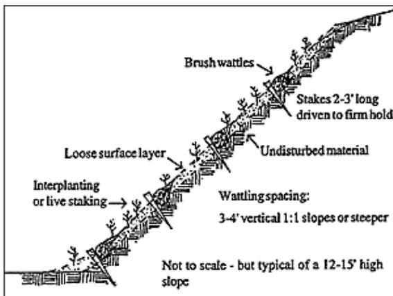
**Figure 4. Slope treatment using wattles and live plants or stakes. Use for loose surface soils with sheet, rill or small gully erosion. (From A.T. Leiser)**
