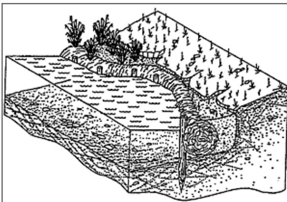
Coir fascines are wattles made from the fibrous outer husk of coconuts. Coir is denser than water so it won't float and is very slow to decay. Coir fascines are a readily available manufactured product and are popular for streambank and wetland restoration where a natural look is desired (*Figure 3*). Coir fascines are placed with their tops at the water surface. Live plants can be placed into coir fascines to create a natural look.
