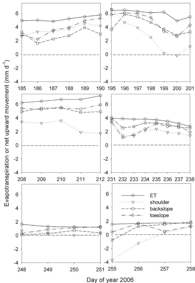
Fig. 6. Selected dry periods showing evapotranspiration and calculated net upward soil water movement for 2006. The different sections are July 4–9, July 14–20, July 27–31, August 19–26, September 5–9, and September 12–15.
