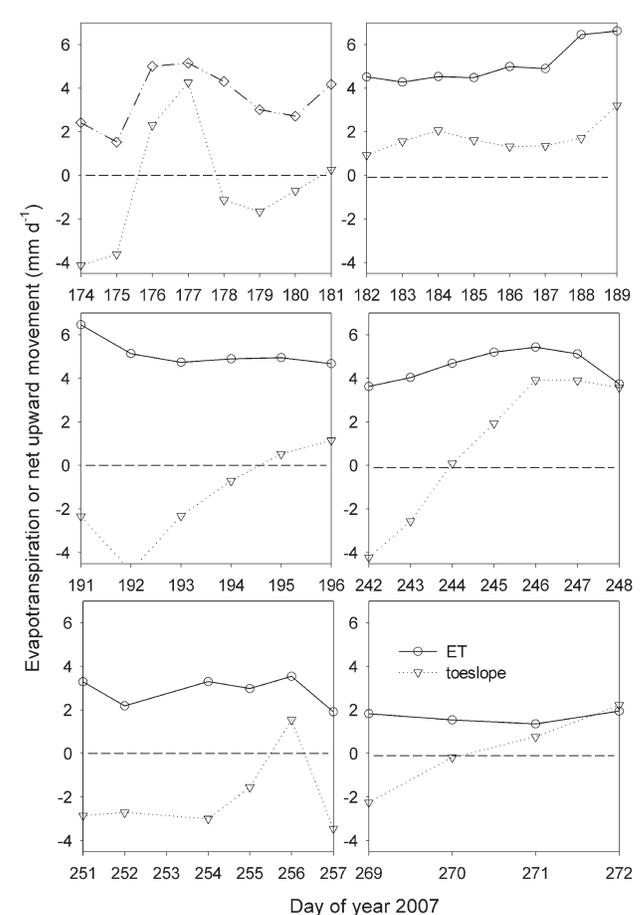
Fig. 7. Selected dry periods showing evapotranspiration and calculated net upward soil water movement for 2007. The different sections are June 23–30, July 1–8, July 10–15, August 30–September 5, September 8–14, and September 20–24.
