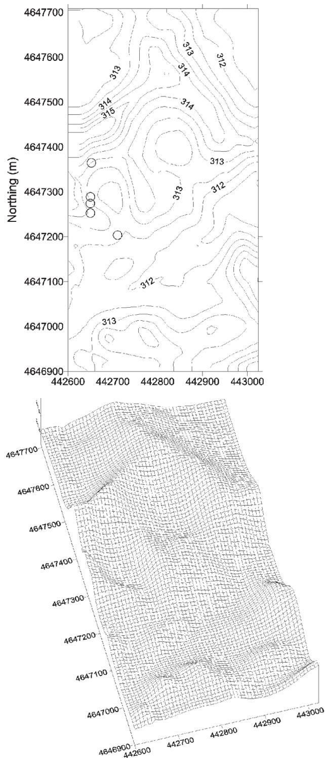
Fig. 1. Field site for 2006 and 2007 data sets. The northernmost point was the site for 2007 (toeslope), and the next points were toeslope, backslope, and shoulder positions in 2006. The southernmost point is the eddy covariance tower and rain gauge. Mean sea elevation is in meters. The contour data is shown below as a wire-mesh diagram to better display the gentle hills and valleys.
