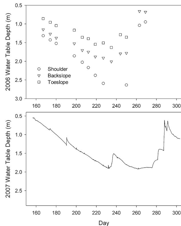
**Fig. 5.** Seasonal water table depths for 2006 shoulder, backslope, and toeslope positions, and for toeslope position in 2007. The date of the x axis is from June 9 to October 7 (152–304).
