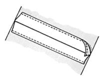
The edge stitch is the simplest finish to apply. Straight stitch 1/8" to 1/4" from the raw edge. An attachment (edge-stitcher) is available for many sewing machines to make this stitching easier.
