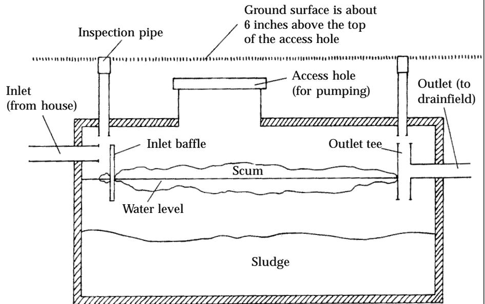
Figure 2. The parts of a septic tank.
