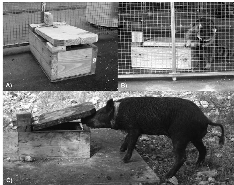
**Figure 1.** (A) Resistance assessment bait station (RABS) propped open with a temporary block. (B) A captive raccoon attempting to open the lid of a RABS in July 2014, National Wildlife Research Center, Fort Collins, CO, USA. (C) An invasive wild pig opening the lid of a RABS in August 2014, Kerr Wildlife Management Area, Hunt TX, USA.
