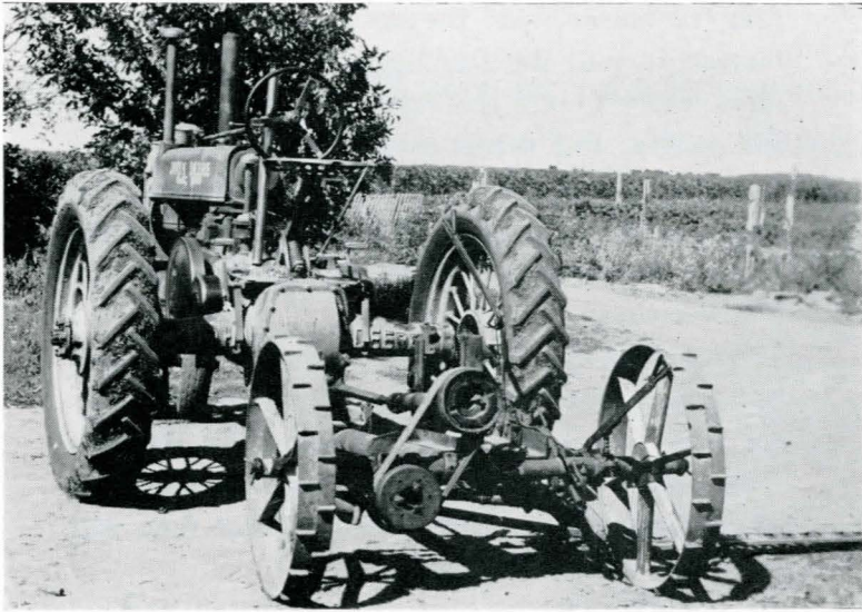
Figure 3. —This mower conversion built by Robert Erickson of Funk, Nebr., uses a flat belt drive from pulley on power take-off drive to pulley on pitman shaft. Pulleys were made from discarded auto brake drums. SINCE UNCOVERED POWER TAKE-OFF SHAFTS ARE VERY HAZARDOUS THEY SHOULD ALWAYS BE COVERED.
