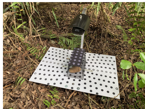
Figure 1. Camera platform comprised of a pattern of circular size standards printed on lightweight sign material, with an inexpensive wide-angle wildlife camera mounted overhead of a live mouse lure chamber, used in a study of brown treesnakes in Guam, USA, 2019–2021.
