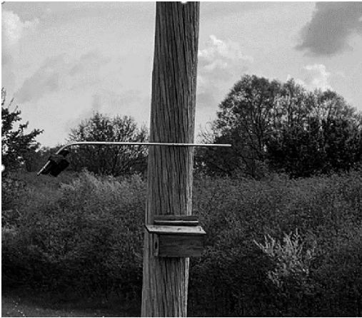
Figure 1. Camera mounting design used during a European Starling nest box study on the National Aeronautics and Space Administration Neil Armstrong Test Facility, Erie County, Ohio, USA, during spring and summer 2021. The mount afforded us ease of camera placement/maintenance and prevented equipment damage or injury to those conducting mowing operations. All 120 nest boxes included the camera mount design, whether the camera was present or not. During spring and summer 2022 we examined the effect of mount relative to enhancing nest predation ( n = 60 nest boxes with the mount; n = 60 nest boxes without the mount).
