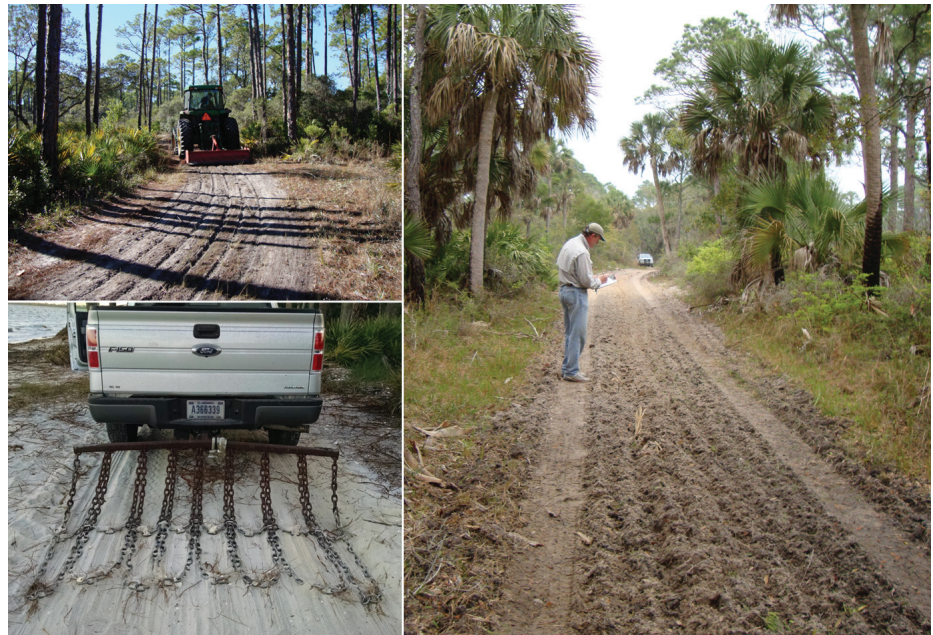
Figure 2. Track plot preparation using a tractor (top left photo); smoothing the track plot surface using a chain drag (bottom left photo); and reading the track plot (right photo)
