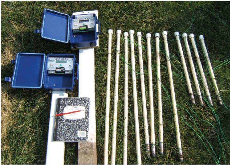
Figure 2. Watermark sensors attached to PVC pipes to be installed at different depths.
