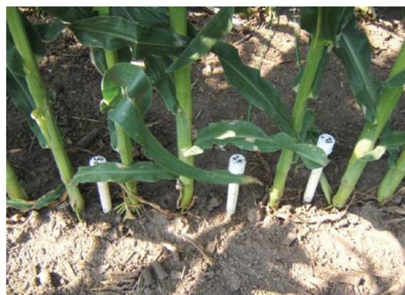
Figure 4. Watermark sensors installed at 12, 24 and 36-in. depths in center-pivot irrigated corn field.
