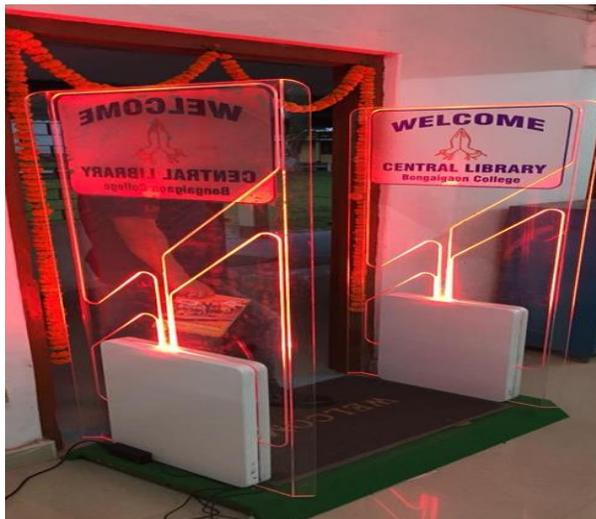
Fig 8: RFID security gate
