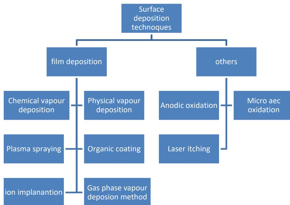
Figure 1 Surface modification techniques for surface hardening
