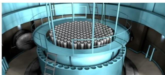
**Figure 3.** The reactor core contains uranium materials in the form of bars, water moderators, and cadmium control bars.
