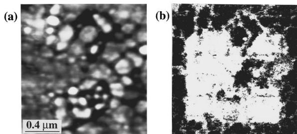
FIG. 5. Simultaneously obtained (a) topographic and (b) piezoresponse images of the fatigued PZT/Pt heterostructure. The bright square of  $1 \times 1 \mu\text{m}^2$ , produced by moving the SFM tip while applying a negative 15 V dc voltage, represents a negatively polarized region. Unswitchable crystallites appear as dark areas inside the white square region.
