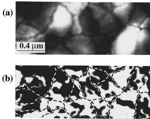
FIG. 1. Simultaneously obtained (a) topographic and (b) piezoresponse images of the PZT/RuO<sub>2</sub> film. White and black regions on the piezoresponse image correspond to negative and positive domains, respectively. Dashed black-white lines in (b) represent grain-boundary contours obtained from the topographic image (a).
