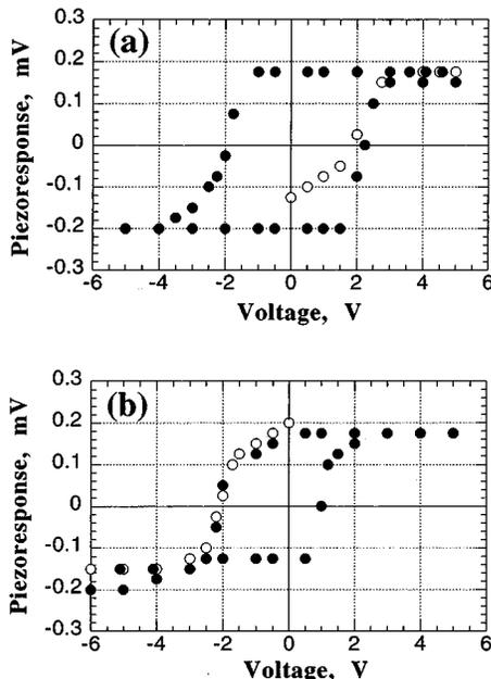
FIG. 2. Piezoresponse hysteresis loops for (a) negative and (b) positive domains in the PZT/RuO<sub>2</sub> film. Open circles illustrate initial parts of the hysteresis loops.
