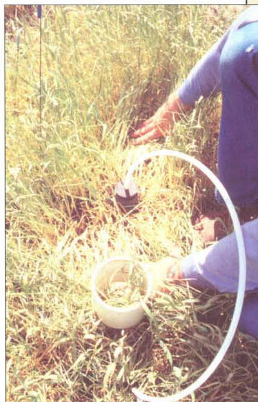
This is one of a number of sites within the corn and alfalfa plots where a vacuum line runs into a tube extended into the root zone for pulling samples of water moving through the root zone for determining nutrient leaching under different rates of effluent application.
