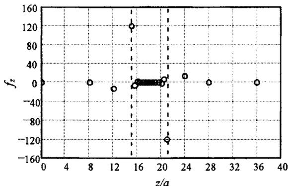
FIG. 4.  $z$  component of “ghost force” on node (atom) vs  $z/a$  for system I (see Table I), in which atoms are in configuration of perfect crystal at  $T=0$ . The vertical dotted lines define regions (see Fig. 2). Discrete points plotted at positions of atoms or nodes.
