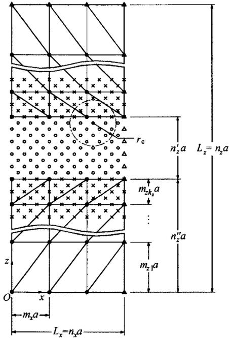
FIG. 1. Schematic side view (in positive  $y$  direction) of Lennard-Jones (12,6) crystal. Atoms depicted in equilibrium positions at  $T=0$  K in near region (inner slab) by open circles and in far regions (outer slabs) by crosses; nodes in far regions represented by filled circles. The open triangles on top and right boundaries signify periodic images of atoms (nodes).
