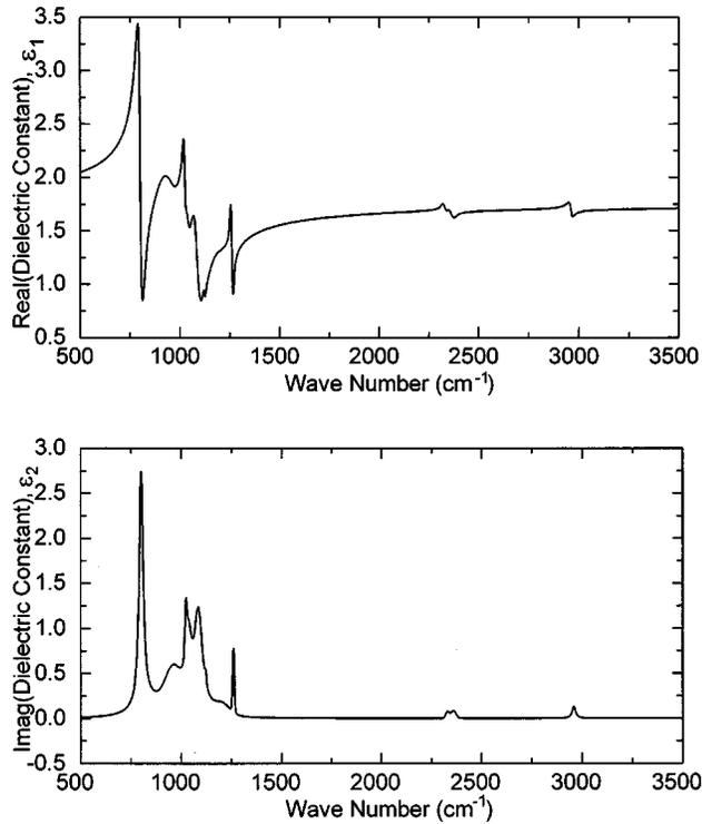
FIG. 5. CV-1144-O optical constants in the IR range.
