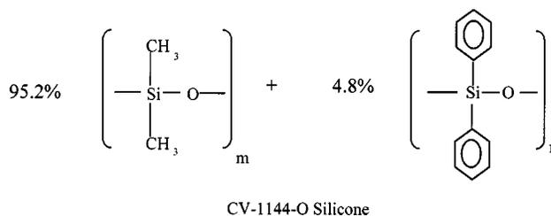
FIG. 1. CV-1144-O chemical structure.
