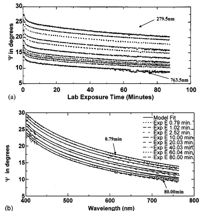
Fig. 7. *In situ* spectroscopic ellipsometry raw  $\Psi$  data obtained from sample 2T, vs (a) exposure time for wavelengths from 279.5 to 763.5 nm and (b) wavelength, for exposure time from 0.79 to 80 min.
