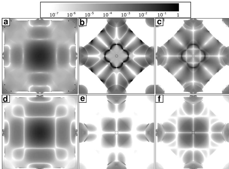
FIG. 2. Transmission probability as a function of  $k_{||}$ . (a)–(c), Fe/MgO/Fe junction with 4 MgO ML; (d)–(f), same junction with Ag interlayers; (a) and (d), majority spins; (b) and (e), minority spins; (c) and (f), antiparallel configuration (per spin).
