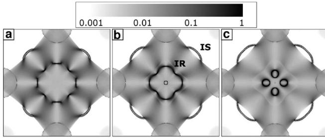
FIG. 1. Normalized minority-spin  $k_{||}$ -resolved DOS at the interfacial Fe layer in Fe/MgO/Fe(001) MTJ for three values of energy: (a) 0.02 eV below  $E_F$ , (b) at  $E_F$ , and (c) 0.02 eV above  $E_F$ . The scale is logarithmic. Interface states and resonances are marked as IS and IR in panel (b).
