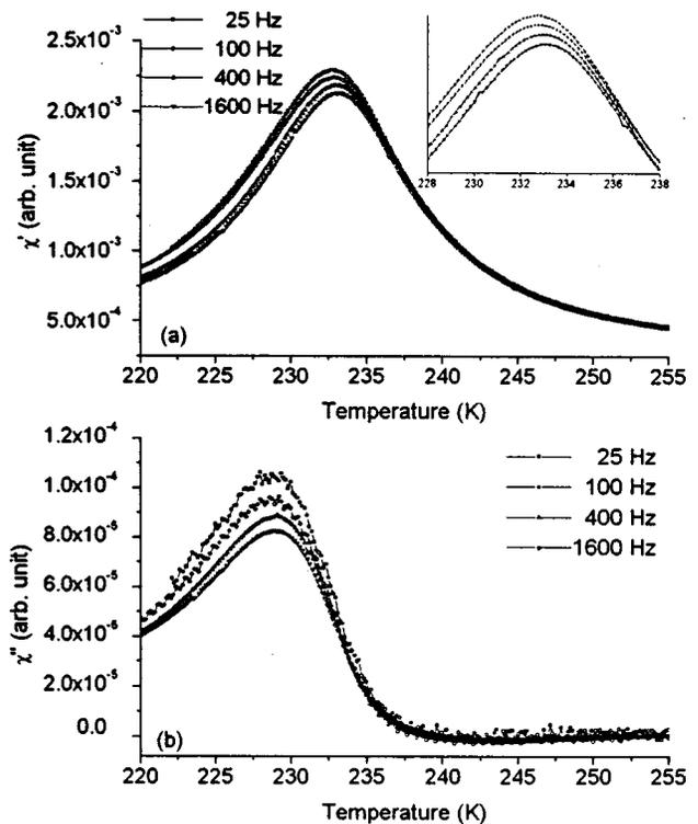
FIG. 3. Frequency dependence of in-phase (a) and out-of-phase (b) ac susceptibility of  $\text{PrCo}_{3-x}\text{Si}_x$  for  $x=0.17$  and  $\nu=25, 100, 400,$  and  $1600$  Hz. The inset shows the cusps in more detail.
