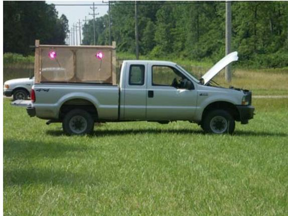
In identifying pulse rate as a critical piece of this puzzle, we refined our pulse capability by refining the Pulselite unit to operate an incandescent lamp to 30 Hz with distinct pulse control.
