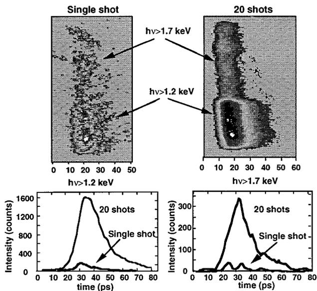
FIG. 5. Streaked images of the broadband x-ray emission from Ni target passing through  $25\ \mu\text{m}$  (cutoff energy  $h\nu > 1.2\ \text{keV}$ ) and  $50\ \mu\text{m}$  (cutoff energy  $h\nu > 1.7\ \text{keV}$ ) Be filters and corresponding line outs for the single shot and 20 accumulated shots. Signal-to-noise ratio is significantly improved after averaging 20 shots.
