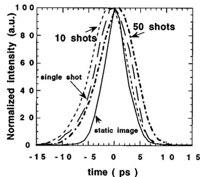
FIG. 4. Experimental data line outs showing  $\pm 1 \text{ ps}$  jitter with direct laser illumination of the gold photocathode of the streak camera.
