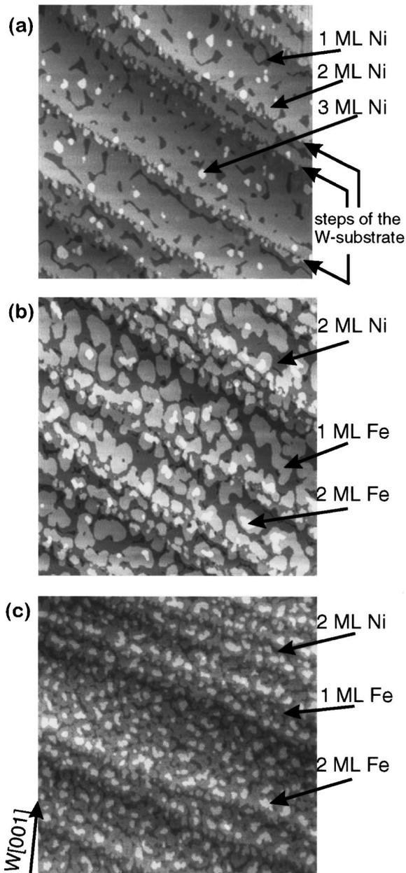
FIG. 1. STM images of Ni/W(110) and Fe/Ni/W(110). Image size is 250 nm $\times$ 250 nm. Terraces of the W substrate, separated by monoatomic steps running from the upper-left to the lower right hand side of the images are apparent. (a) Deposition of 2 ML Ni on W(110). Anneal at 900 K after deposition of the first ML Ni. (b) Deposition of 0.8 ML Fe on (a) at 300 K. (c) 0.8 ML Fe on 2 ML Ni/W(110). First Ni layer not annealed. Note the considerably increased island density compared to (b).
