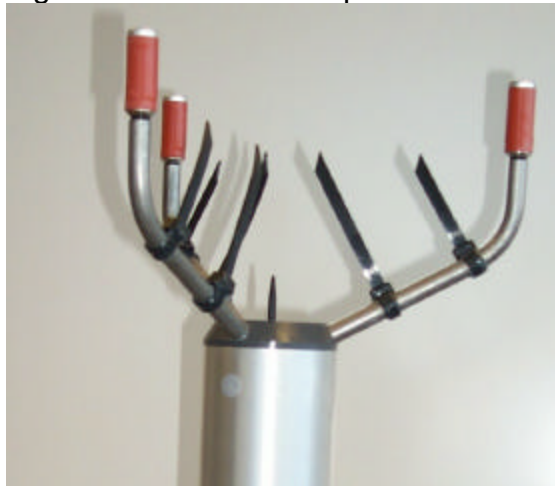
Figure 11. FAA Tie Wrap Solution
