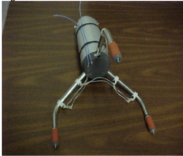
Figure 12. Notional Electric Fence Mock-up
