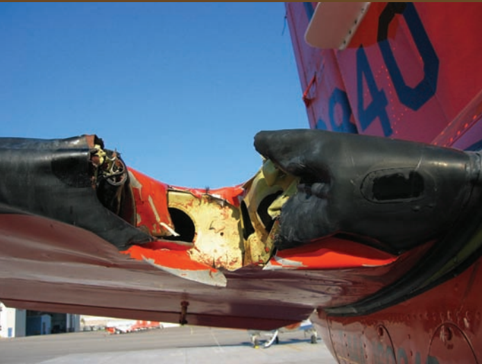
Figure 1 —Bird strikes affect both civil and military aircraft: this Navy plane collided with a single turkey vulture in Florida.
