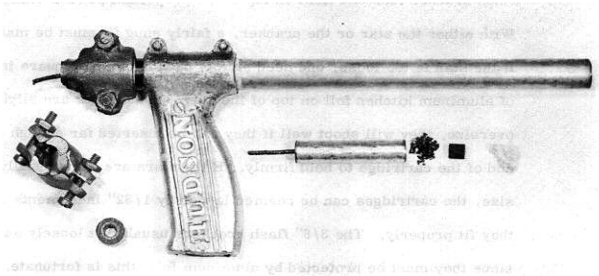
Figure 14 - Hand Mortar for 3/8" Stars and Crackers. The Barrel Is 12" Long with 3/4" O. D. and 5/8" I. D. The Handle Is a Standard Hudson Sprayer Part and the End Plug Is a Spray Hose Clamp. The Clamp Can Be Removed Easily to Clean the Barrel. The Cartridge Is a 2" Piece of Water Pipe 1/2" O. D. and 3/8" I. D. One End of the Cartridge Is Plugged with Solder and Drilled to Take the Fuse. The Powder Charge Which May Be from 1/2 to 1 gm Is Placed in the Cartridge Followed by the Star and a Bit of Rock Wool or Aluminum Foil Wadding. The Cartridge Is then Dropped in the Mortar and the Fuse Lighted.
