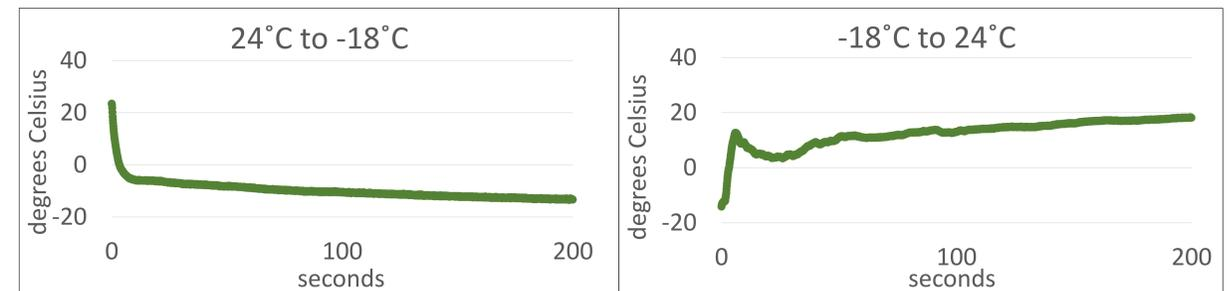
Figure 4: Response time of the thermistor. Effect of wind is visible in right-hand plot.
