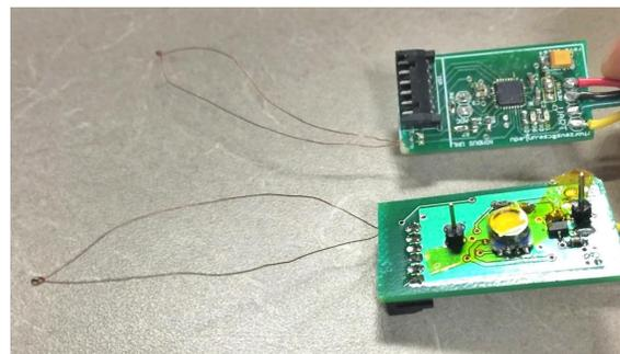
Figure 3: The fully assembled circuit board for sensing temperature
