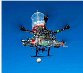
Figure 2: The fireball dropper UAV in action
