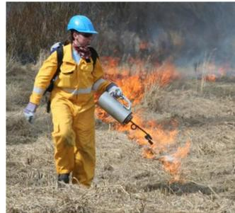
Figure 1: The drip-torch method currently used for starting controlled burns
