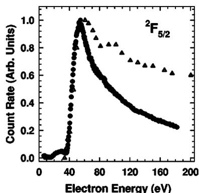
FIG. 4. Optical excitation functions for the  ${}^2F_{5/2}$  state. Solid circles: data of this work, taken with a target pressure of 3.0 mTorr, monitoring the 463.73 nm transition. The intensity is measured through a linear polarizer set at an angle of  $54.8^\circ$  with respect to the beam axis [42] so that it does not depend on the alignment of the excited state. Open triangles: data of Ref. 9 for the 458.90 nm transition, taken with pressure between 0.7 and 5 mTorr (see text).
