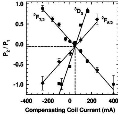
FIG. 5. Ratio of polarization fraction  $P_2$  to the total linear polarization  $P_1$  vs  $I$ , the current through the compensating Helmholtz coils.  $P_2$  for zero  $B$  field in the collision volume must equal zero. Data for  ${}^2F_{7/2}$  (circles) and  ${}^2F_{5/2}$  (diamonds) transitions in Ar II, as well as the  ${}^3D_3$ - ${}^3P_2$  811.5 nm transition (squares) in Ar I (see text).
