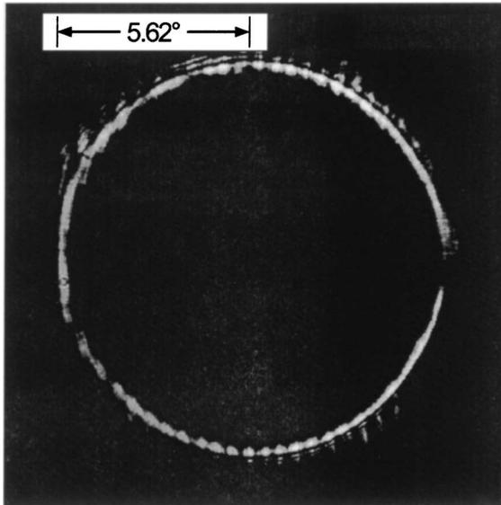
FIG. 3. Angular pattern of the third harmonic generated for a plasma density of  $3 \times 10^{19} \text{ cm}^{-3}$  and a pump laser intensity of  $1.7 \times 10^{17} \text{ W/cm}^2$ , when a prepulse is used.
