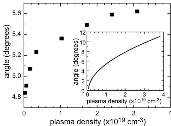
FIG. 4. Angle (radius) of the cone of emission for the narrow unshifted third harmonic as a function of plasma density at a laser intensity of  $1.7 \times 10^{17}$  W/cm<sup>2</sup>. The error is indicated by the size of the symbols. The inset shows the theoretical prediction that uses Eq. (1).
