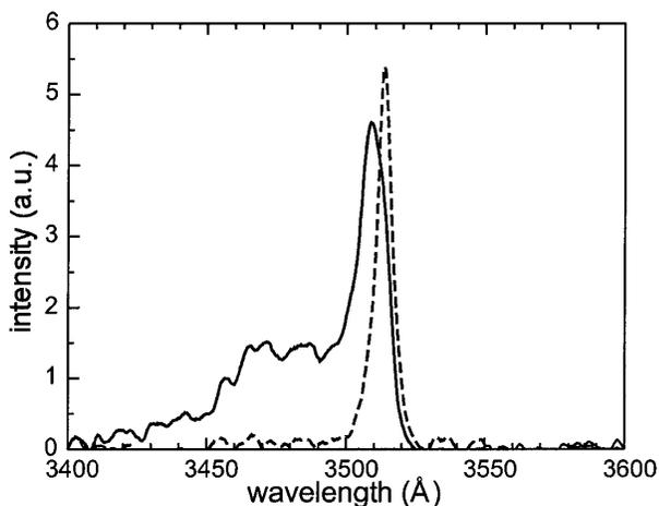
FIG. 1. Spectra of the third harmonic generated in helium for  $3 \times 10^{19}$  cm<sup>-3</sup> gas density and  $1.5 \times 10^{17}$  W/cm<sup>2</sup> pump laser intensity with (dashed line) and without (solid line) the prepulse.
