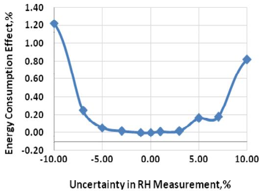
**Figure 4** Uncertainties in RH Measurement on Energy Consumption
