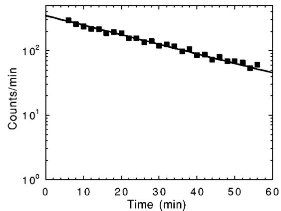
FIG. 3. Measured decay of radioactivity vs the time for the  $^{10}\text{B}(d,n)^{11}\text{C}$  reaction (squares). The solid line corresponds to the theoretical result and demonstrates  $\sim 20$  min half-life of  $^{11}\text{C}$ .
