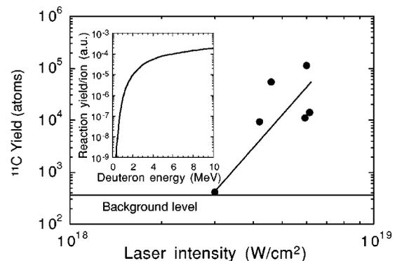
FIG. 4. Experimental yield of  $^{11}\text{C}$  vs the laser intensity for the  $^{10}\text{B}(d,n)^{11}\text{C}$  reaction. The inset shows calculated yield of  $^{11}\text{C}$  per one deuteron as a function of energy cutoff  $E_{\max}$  for a uniform distribution of deuterons in energy space.
