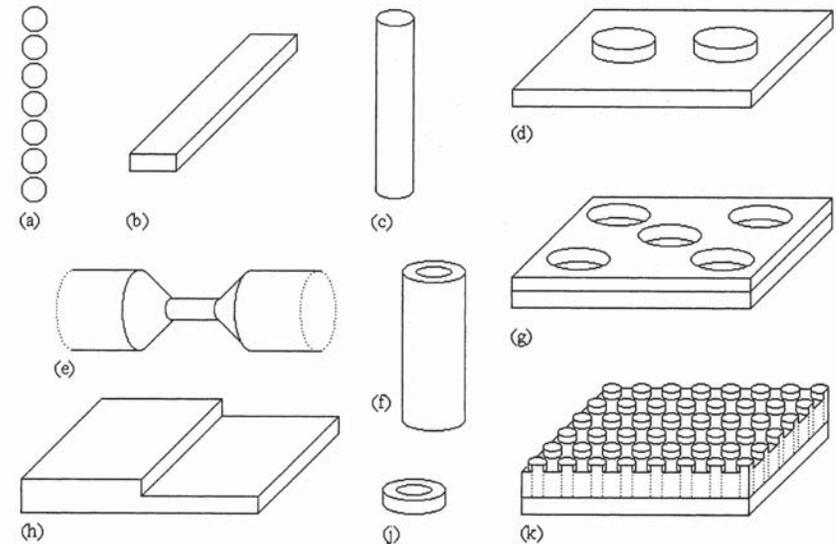
**Figure 1.** Typical nanostructure geometries: (a) chain of fine particles, (b) striped nanowire, (c) cylindrical nanowire, (d) nanodots, (e) nanojunction, (f) nanotube, (g) antidots, (h) vicinal surface step, (j) nanoring, and (k) patterned thin film. Note that the figures can consist of multilayered and granular nanocomposites.
