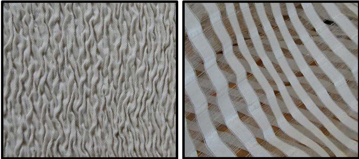
Long Staple, Egyptian Giza cotton, Merino Wool. Pleating created via differential shrinkage, left..
