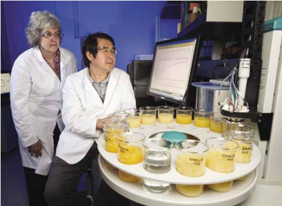
Horticulturalist Elizabeth Baldwin (left) and chemist Jinhe Bai review data from the “electronic tongue,” a device that can detect chemical differences related to taste to see whether it can distinguish between juice from HLB-infected oranges and from noninfected oranges.
