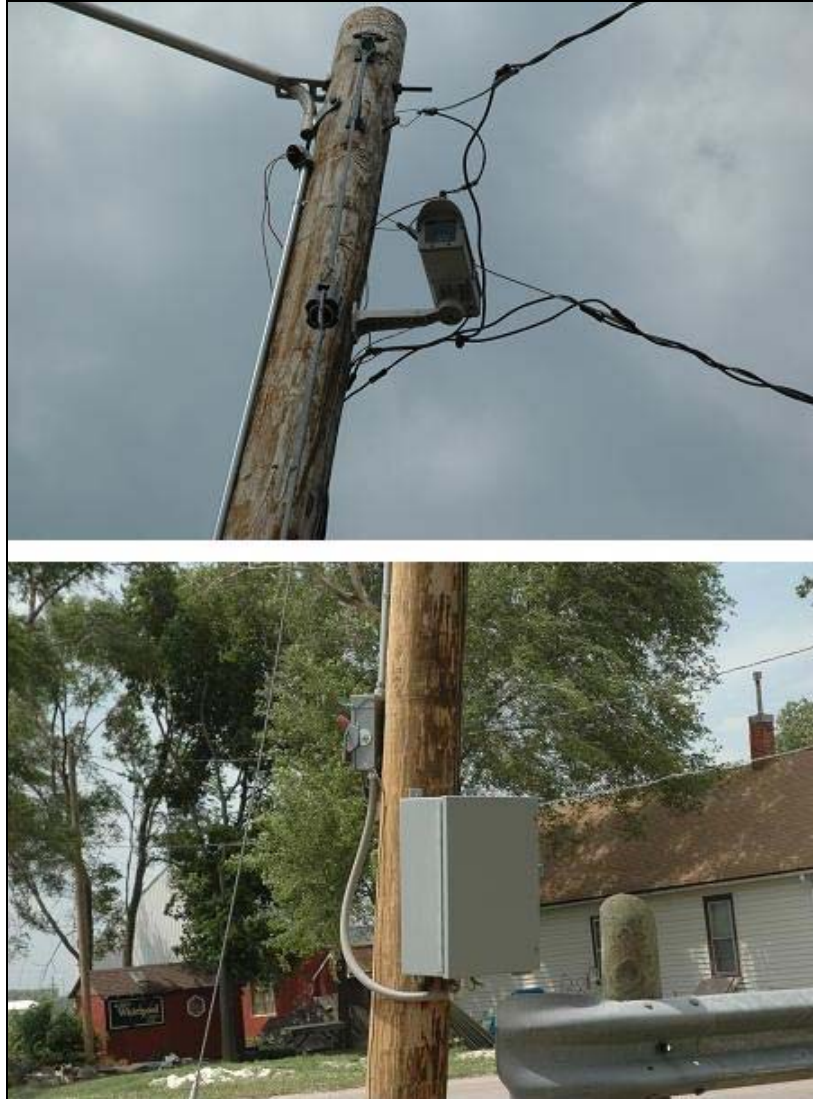
Figure 3.4. Day and night vision camera and DVR storage box mounted on a utility pole in Fremont, NE
