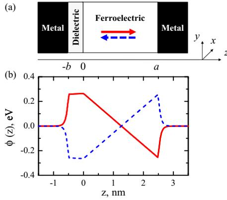
FIG. 1. (Color online) Geometry (a) and the electrostatic potential profile for the two opposite polarization orientations (b) of a FTJ:  $a=25$  Å,  $b=5$  Å,  $\epsilon_d=300$ ,  $\epsilon_f=90$ ,  $\delta=1$  Å, and  $P=20$   $\mu\text{C}/\text{cm}^2$ .
