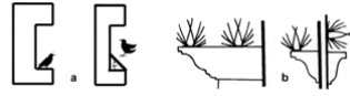
Figure 3. A board or metal covering over a ledge at a 45° angle (a) or porcupine wires (b) can be used to prevent roosting and nesting.
