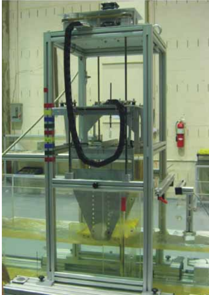
Figure 13. Photo. Deck force analyzer system at the TFHRC hydraulics lab.
