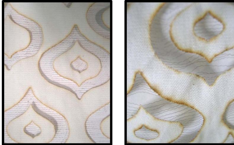
**Figure 11.** Raster cut through a woven cotton textile with a weft inserted fine metal weft thread.
