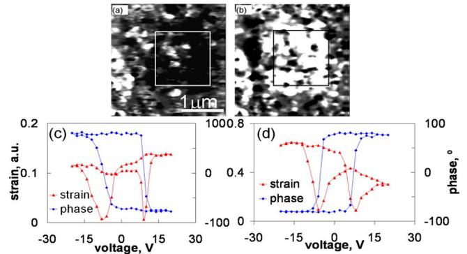
FIG. 3. (Color online) Piezoresponse images of the PZT52/48 film showing domain structures after (a)  $-15$  V and (b)  $+15$  V dc poling, respectively. Local piezoresponse hysteresis loops were obtained in (c) inversely poled grains and (d) in the normally switched region.
