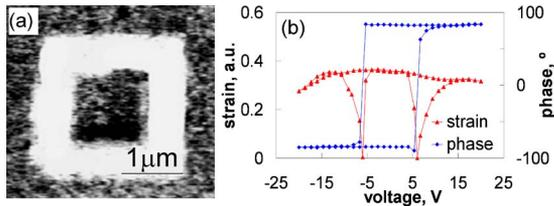
FIG. 1. (Color online) (a) PFM image and (b) piezoresponse hysteresis loop obtained on bare surface of the PZT20/80 film. The bright and dark areas in (a) are poled by dc biases of +10 and  $-10$  V, respectively.
